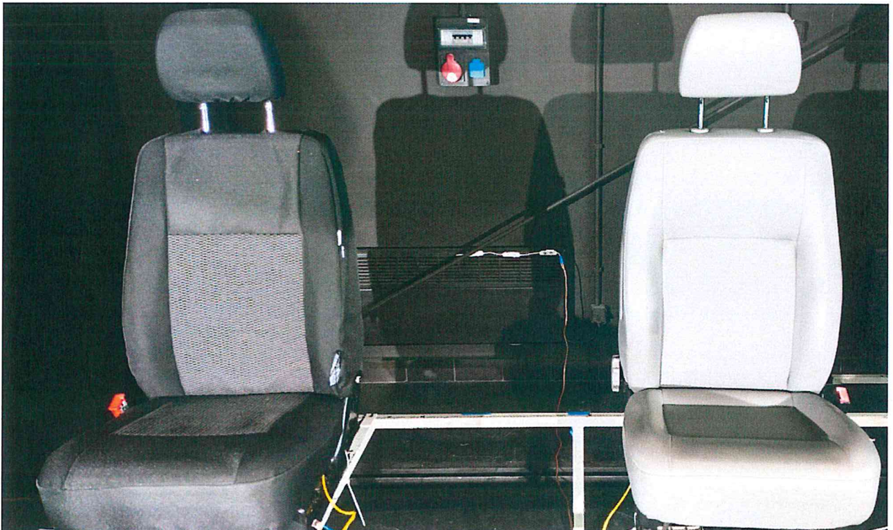
Fot. 1. Obiekt badań – pokrowiec typu AirBag, model Tailor Made (po lewej stronie) Photo 1. Test object - cover AirBag type, model Tailor Made (on the left)
